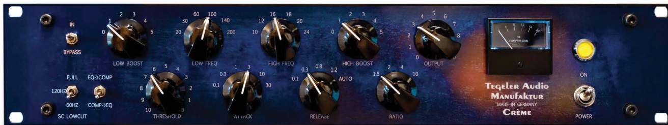
Crème has a dedicated EQ section with 5 LF and 6 HF frequency choices (boost only).
