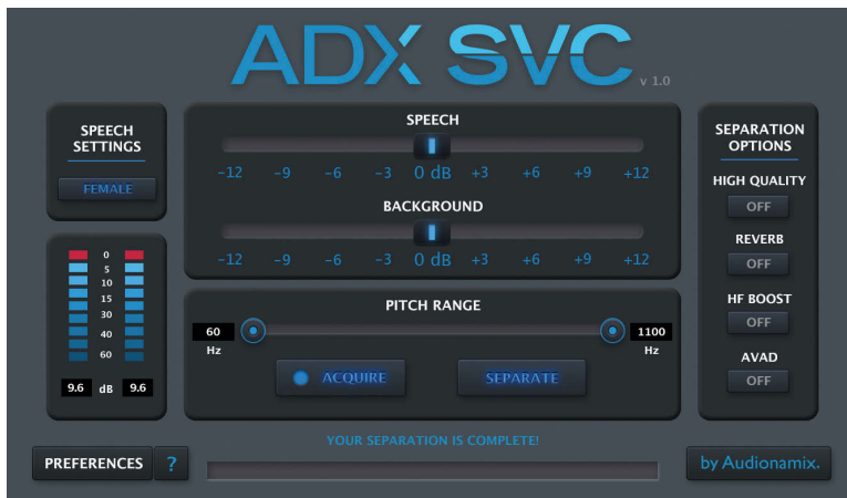
ADX SVC's simple, user-friendly GUI interfaces with intensive, cloud-based processing to separate speech from background noise. The Separation Options (on the right side of the GUI) affect the quality and content of the extraction.
